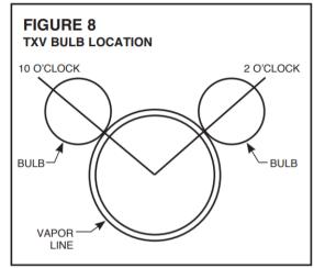
3.3 TXV SENSING BULB (TXV COILS ONLY) IMPORTANT: DO NOT perform any soldering with the TXV bulb attached to any line. After soldering operations have been completed, clamp the TXV bulb securely on the suction line at the 10 to 2 o'clock position with the strap provided in the parts bag. (See Figures 7 & 8)
